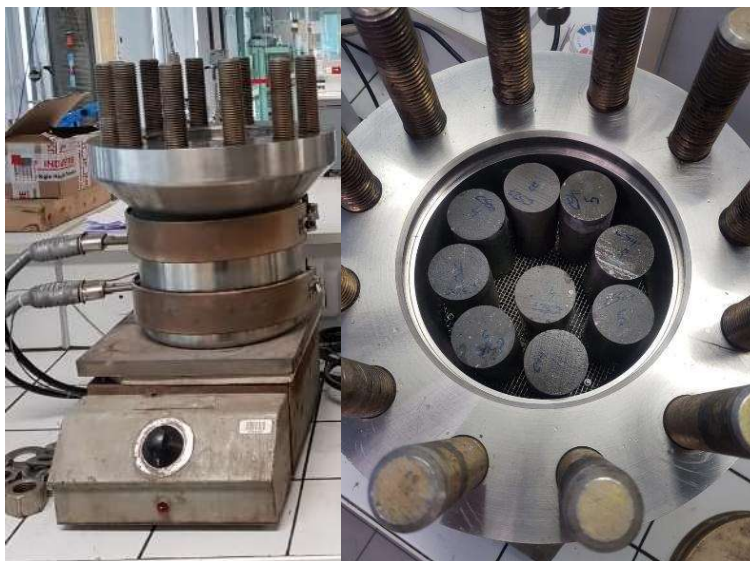
Fig. 1: Cell used for subjecting cement samples to CCS conditions
